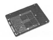
This is a standard-issue 2.5" LAPTOP hard disk drive, and it is ALSO an (SSD/SOLID-STATE DRIVE). What SEPARATES an SSD from a MECHANICAL DISK DRIVE, is the fact that a SOLID STATE DRIVE has NO MECHANICAL PARTS IN IT that:
